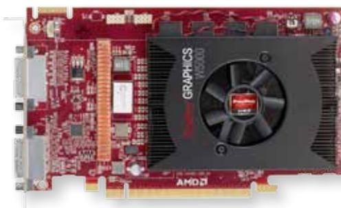
can support a variety of medical imaging workflows. It can drive up to two 5MP displays independently or combined, or a drive a single 10MP display with dual input connectors as a single large desktop. Images and scans can also be viewed at a maximum resolution of 2560x2048 (in packed pixel mode), allowing professionals to see in greater detail.
